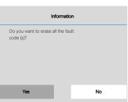
After reading the retrieved codes and making appropriate vehicle repairs, use this function to clear fault code.
