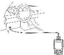
Connection To connect the main unit with the main cable To get power supply from the car via OBDII-16
