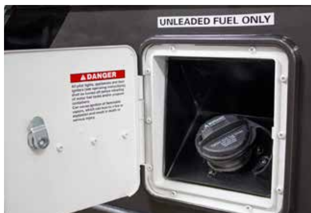
Fuel Tank Inlet for Fuel Transfer System
