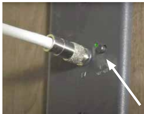
Antenna/Cable push-button selection switch with green LED
