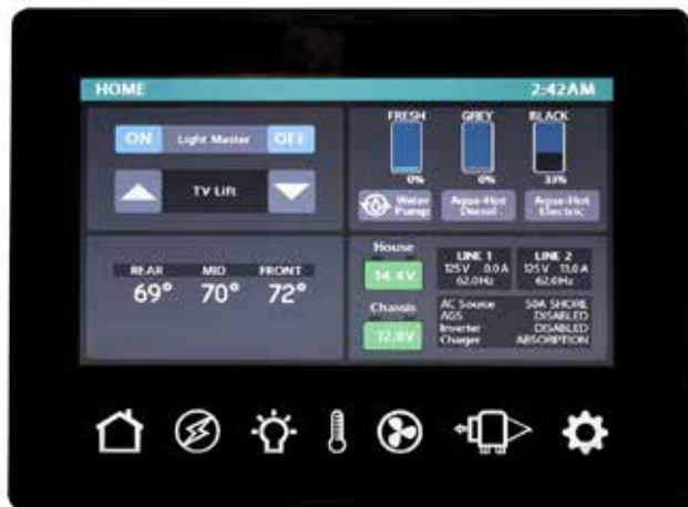
Typical multiplex main control panel. Electrical system monitoring is usually located on the main menu (Home) screen.
