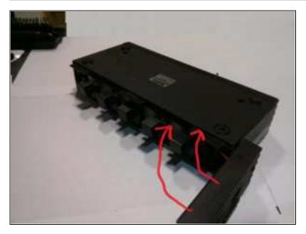
Snap the front panel back into place and re-insert the 3 front panel screws, completing the replacement.
