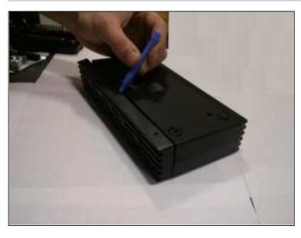
Carefully pry off the front panel of the device to reveal the button in need of replacement.
