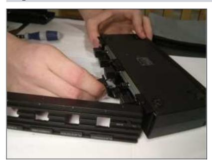
• Push the replacement button into its new housing.
