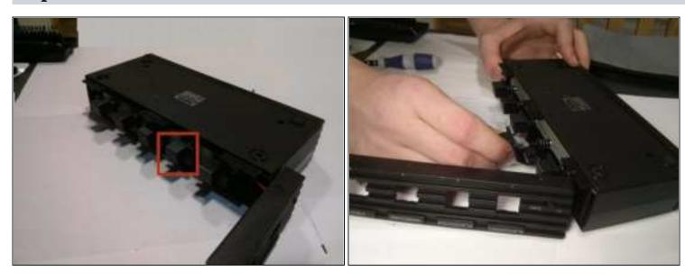
• Pull firmly on the button in need of replacement to free it from its housing.
