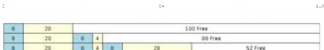
Fig. 33: Sending items to No-Split or Allow-Split ring buffers
