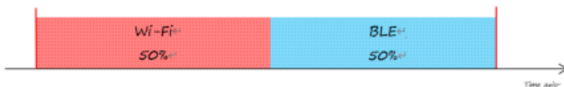
Fig. 98: Time Slice Under the Status of Wi-Fi CONNECTED and BLE CONNECTED
