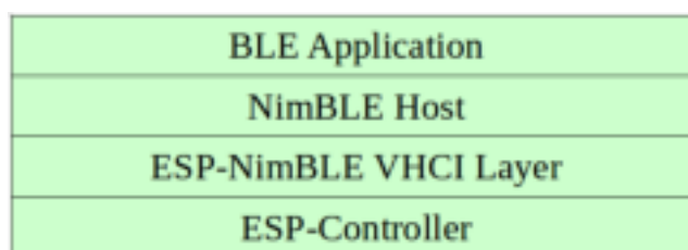
Fig. 1: ESP NimBLE Stack
