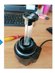
Carefully remove the UV lamp by pulling it upwards. Remove the black rings at the top and base of the lamp.
