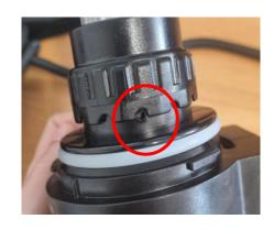
Tighten the black ring until you feel resistance, making sure the screw hole is accessible through one of the ring's notches.
