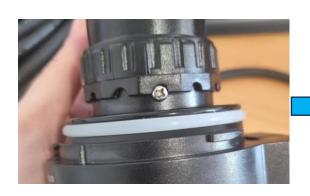
Unscrew the small screw that secures the clamping ring.
