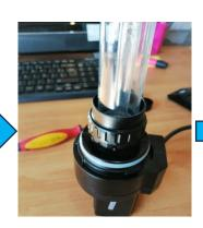
Unscrew the ring and slide it upwards.
