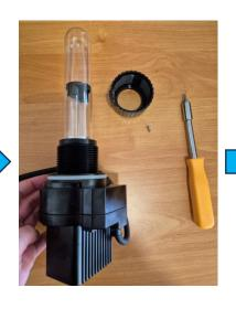
Unscrew the ring and take it out by sliding it to the top of the lamp.
