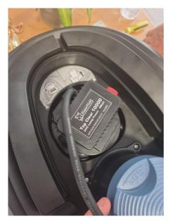
Turn the block clockwise. At the point shown in the photo, you'll feel resistance as the notches make contact. Press firmly on the block so that its entire base is in contact with the housing, then continue turning to the right until you hear a click.
