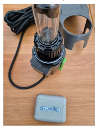
Place a magnet (strong enough, in this case an aquarium cleaning magnet) on the flat side of the ballast: the lamp will then light up.
