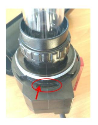
Using a FLAT, NON-SLIP tool (to avoid damaging the membrane), press the membrane into the notch at the point indicated on the left: the lamp will light up.
