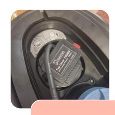
Pull up the red lock, then turn the UV head on the left (counterclockwise)
