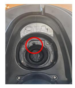
Once correctly reassembled, insert the UV block into its housing. With the safety catch (plastic nipple) facing you, insert the block slightly turned to the left, with the red lock on the right.
