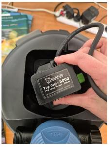
Turn the block clockwise. At the point shown in the photo, you'll feel resistance as the notches make contact. Press firmly on the block so that its entire base is in contact with the housing, then continue turning to the right until you hear a click.
