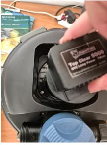
Once correctly reassembled, insert the UV block into its housing. With the safety catch (round magnet) facing you, insert the block slightly turned to the left, with the green lock on the right.
