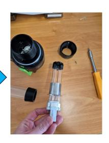
Carefully remove the UV lamp by pulling it upward. Take out the black ring and the metal ring.
