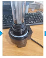
Carefully remove the quartz by pulling it upwards.
