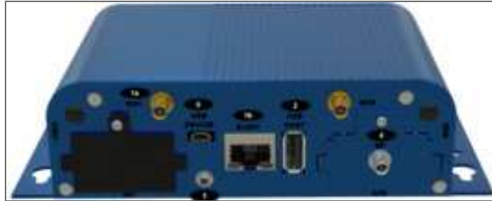
Figure 6-3: Multitech Conduit Gateway rear view connectors illustration
