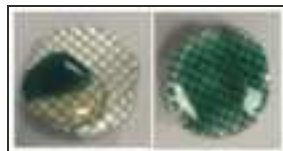
Figure 5-7: Applying adhesive on the flat face of the epoxy mount adapter
