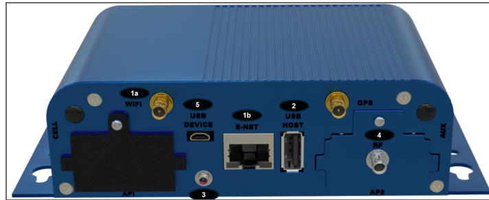
Figure 6-3: Multitech Conduit Gateway rear view connectors illustration
