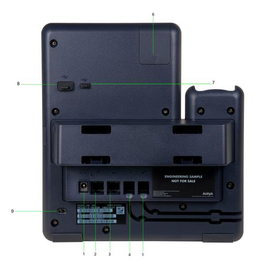
The image schematically describes which device to connect to which jack.
