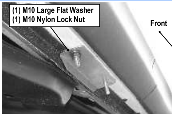
(Fig 9) Locking Plate (DCS1) Installation (Driver Center Side)
