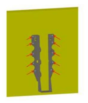
3.Lock the wood square in the support beam hanger with 3 screws on each side.
