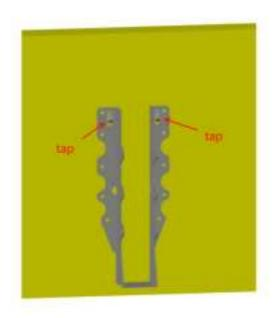
2.10 screws lock the support beam hanger to the beam
