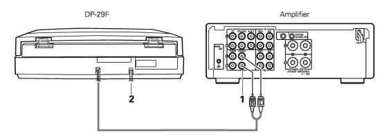
Connect the Left and Right PIN-plugs of the turntable's output cord to your amplifier's PHONO jacks etc.
