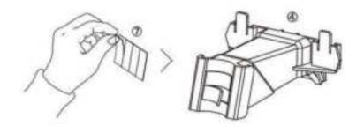
2. Lock the indicators on the bar bracket or seat tube bracket depends on your needs.
