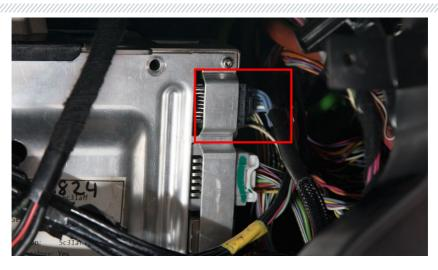
The cable LC007-LY is used in case of MCU with AP3.1 (with port 1000base-T1 (or you can change LC004-L3 so that the interface 100base-T1 connected to pins tuner).
