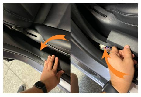
CAN VEH can be connected to the X930 connector located at the back of the center console.
