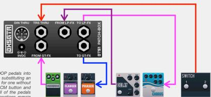
\*\* Instantly re-route the FX LOOP pedals into the front of the amplifier, when substituting an amp with an effects loop (4CM) for one without (2CM), by pressing the 4CM/2CM button and selecting the 2CM position. All of the pedals and all of the pedalboard connections remain unchanged! All of the necessary (color coded) signal path changes are taken care of by/within the OTS1 Patch-Box, automatically.
