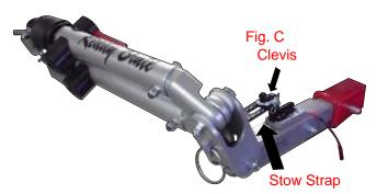
(Note) If RV is to be driven with tow bar in stow position NSA recommends wrapping legs with bungee strap, and hooking leg ends to RV bumper to hold Ready Brute in place over rough roads.
