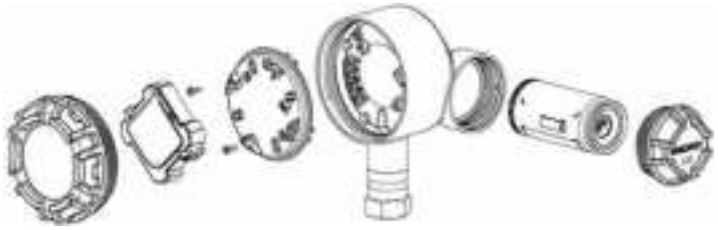
Figure 3-3: Exploded View of LCD Display Assembly
