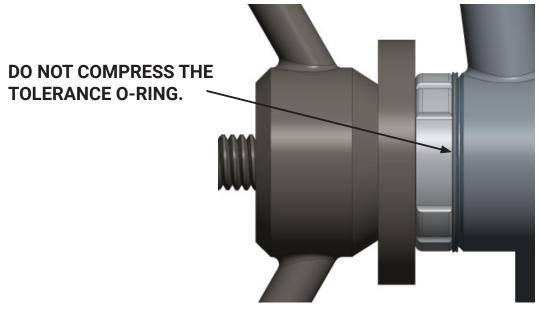
2 Start threading the **Right/Drive Cup** in **CLOCKWISE** with your M30 BB tool. As it threads in, you will feel friction build as the Orange Rubber Collet expands inside the frame. **This is normal. Grab your second BB tool at this point**
