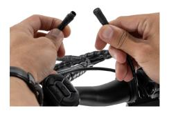
5. To plug in the display, align the arrows on female and male side of the green display plugs.
