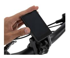
Ensure the display locks in place to the tabs. These tabs secure the display.
