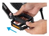
This is what the pedal should look like when correctly installed, with the spring-loaded sleeve fully seated and locked against the crank arm.
