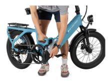
Insert the key at the key port. Turn the key clockwise to the locked position to lock the battery in place. A locking pin will fill the hole on the underside of the downtube.
