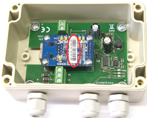
Fig. 6. The MAC address located on the INTRE module.
