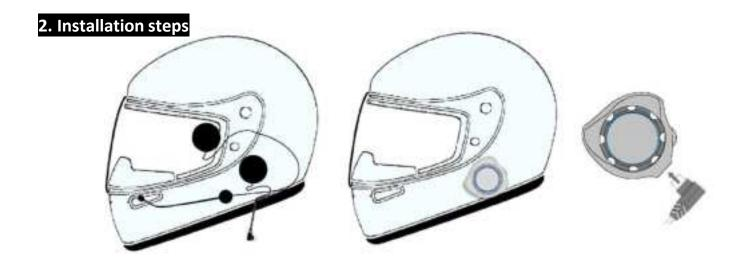
Attach the speakers to the inside of the helmet in the ear position, attach the microphone pole to the left side of the helmet in the proper position, make sure the microphone is in the mouth position, and organize the wiring harness and liner.
