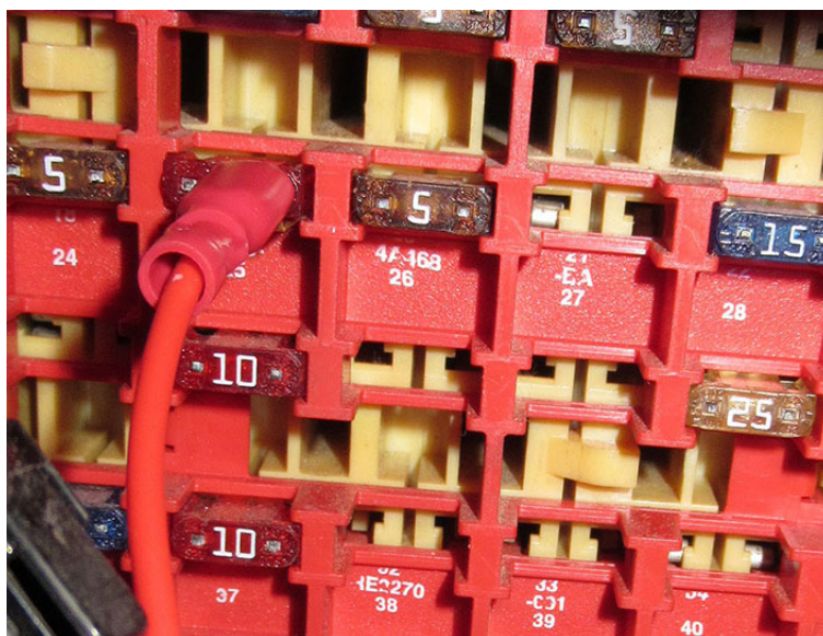
Figure 4 – Reinstall Fuse and Attach Red Wire with Quick Disconnect
