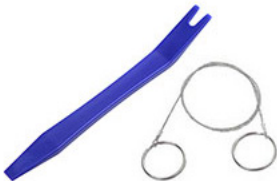
Figure 9 – Tools to Remove Transponder Mounted with Adhesive
