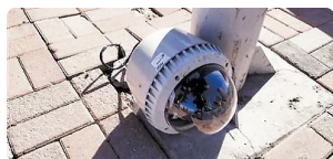
Structural damage of the equipment by vibrations
