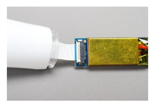
7: Insert the probe into the handle and fix it with screws
