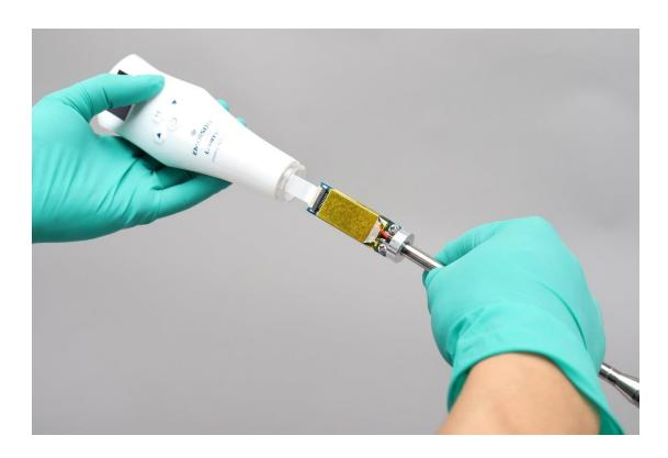
5: Lift the white flip cover of the cable terminal to ninety degrees, and gently pull out the cable
