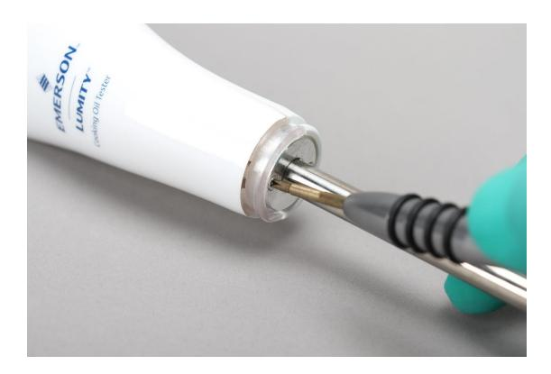
4: Gently pull out the probe rod in the vertical direction until you see the cable terminal
