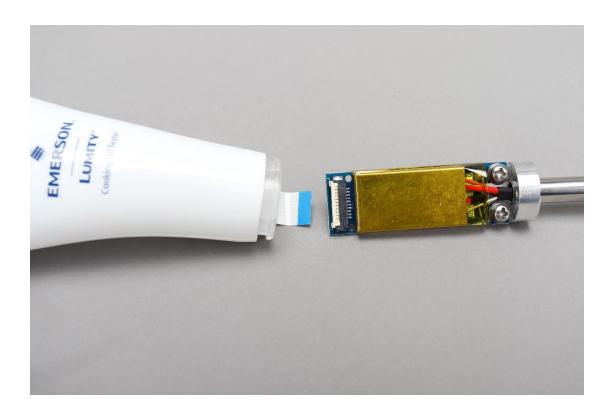
6: Insert the cable into the terminal according to the color shown in the figure, and press down the white cable terminal
