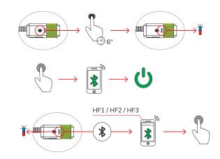
Note: Pairing is a process that only needs to be completed once. When the Twiins® HF device is paired to a specific device, both devices will connect automatically when switched off and on.
