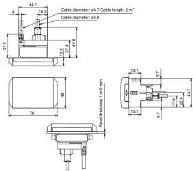
\*1 Cable specification: IL-1000 12 cores, Nominal cross-section area brown/blue: 0.20 mm², others 0.15 mm² : IL-1550 8 cores, Nominal cross-section area: 0.15 mm²
