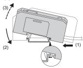
To dismount the sensor, raise the main body in the direction of the arrow (3) while pushing the main body in the direction of the arrow (1).
