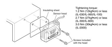
Mounting when detecting targets close to a wall
