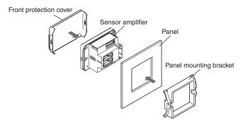
To remove the panel mounting bracket, widen the claws at both ends of the panel mounting bracket using a screwdriver, etc. and remove alternately.
