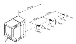
The optical axis may vary by approximately  $\pm 1.5^{\circ}$  (IL-2000), or  $\pm 2.0^{\circ}$  (IL-030/IL-065/IL-100/ IL-300/IL-600).
