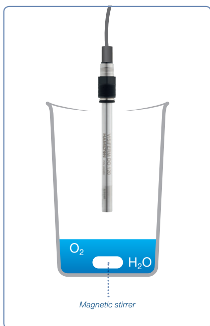
Figure 22: Calibration setup in saturated medium
