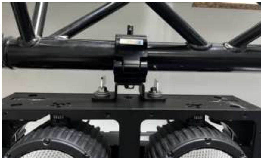
Figure 5. Omega clamp attached to fixture frame
