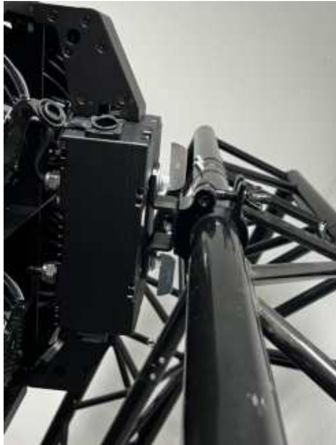
Figure 6. Omega clamp attached to rear of fixture
