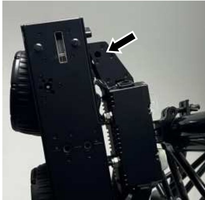
Figure 4. Safety cable attachment point
