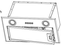
Push the lamp from inside to remove the lamp.
