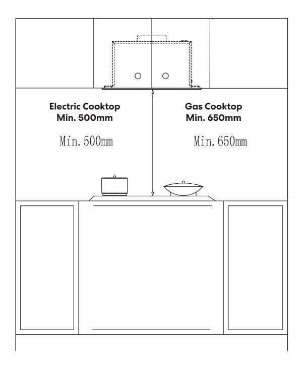
Before installation, make a decision whether you want the air extracted or recirculating. Use the diagram below as reference.
