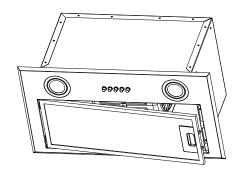
Remove the stainless steel frame by unfastening the 4 screw (M4\*10).
