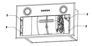
Unfasten the screws (ST4\*10), remove the lid of the terminal box, disconnect the wires to the Commands at the connectors.
