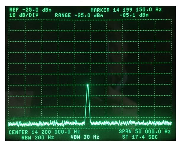
As with any direct conversion transceiver, such as with the Elecraft KX3, the LO radiates out the antenna jack. The above screen shot is through a 30 dB pad, thus when connected to an antenna, the level is -55 dBm with the preamp OFF and the attenuator OFF. The preamp's reverse isolation reduces the LO level 22 dB. The attenuator reduces the LO level 15 dB.
