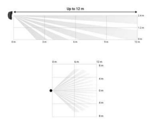
If the detector is not installed at the recommended height, this will reduce the area of the motion detection zone and impair the operation of the function of ignoring animals.
