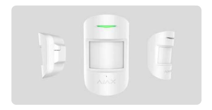
**CombiProtect** is a device combining a wireless motion detector with the viewing angle of 88.5° and distance up to 12 meters, as well as a glass break detector with the distance up to 9 meters. It can ignore animals and detects a person within the protected zone from the first step. The calculated battery life of the detector is up to 5 years from a pre-installed battery. The device is designed for indoor use only.
