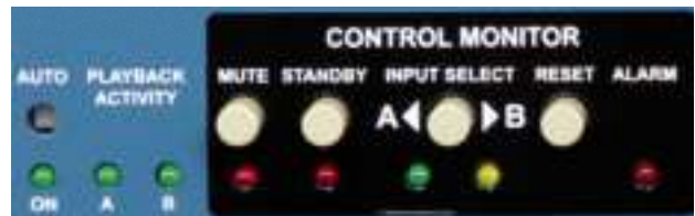
The AUTO-SWITCH controls on the SW8-USB
