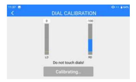
4. Calibration of dial middle points is finished. The next step is to calibrate dial maximum and minimum positions.
