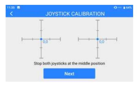
3. According to the tips, if joystick coordinates are not "(0, 0)" when both joysticks are standstill, it shows that joystick middle points are displaced. Please touch "next" and do not touch joysticks.
