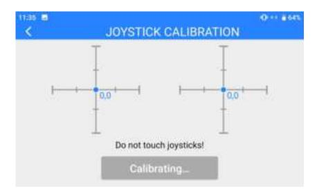
4. Calibration of joystick middle points are finished. The next step is to calibrate joystick maximum and minimum positions.
