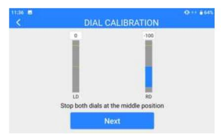
3. According to the tips, if dials' coordinates are not "(0, 0)" when both dials are standstill, it means that dial middle points are displaced. Please touch "next" and do not touch the dials.
