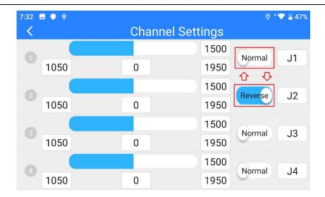
Select a target channel. Then touch the "Normal" or "Reversed" button. It's done.
