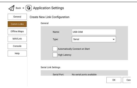
Confirm and start to "Connect". The top progress bar in QGC starts to move, which means the remote controller is communicate with QGC automatically.
