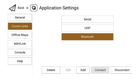
4. Confirm and start to "Connect". The top progress bar in QGC starts to move, which means the remote controller is communicate with QGC automatically. Please wait until the datalink connection is established.
