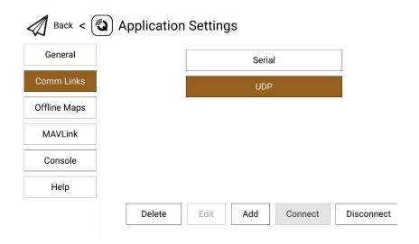
5. Confirm and start to "Connect". The top progress bar in QGC starts to move, which means the remote controller is communicate with QGC automatically. Please wait until the datalink connection is established.
