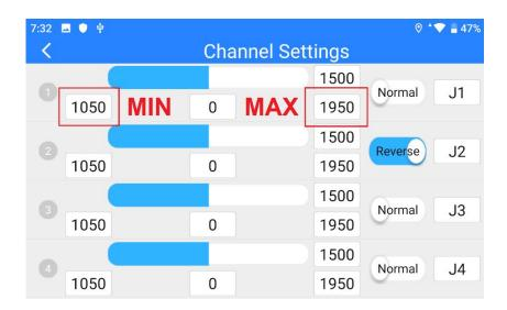
Select a target channel and input your required maximum or minimum channel value. It's done.
