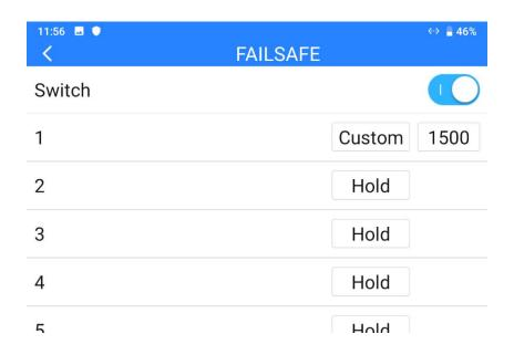
5. After configuration, the channel would output the value if the air unit lost communication with the ground unit during flight.
