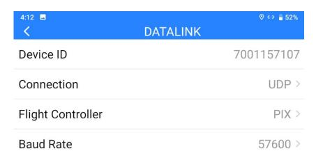
2. Run Mission Planner, select the relevant port (UDPCI) and match the baud rate. "Port" as "19856". "Server addresses" as "192.168.144.12". Then connect.
