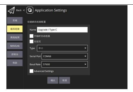
4. Confirm and start to "Connect". The top progress bar in QGC starts to move, which means the remote controller is communicate with QGC automatically. Please wait until the datalink connection is established.
