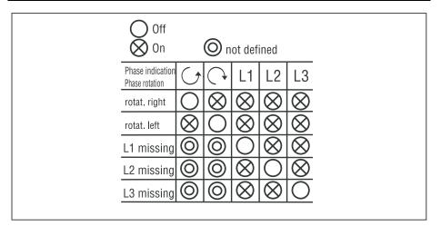
Figure 2. Phase Indication Table (shown on the rear of the 9062)
