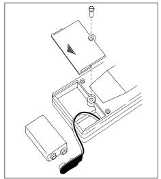
Figure 4. Battery Replacement
