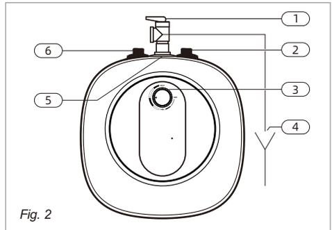
1. Temperature & pressure relief valve, 3/4 NPT male
