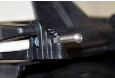
Fig. 256: Fixed position, i.e. the monitor cannot be tilted.
