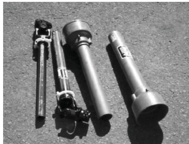
Disassembled Fig. 36 DRIVELINE COMPONENTS
