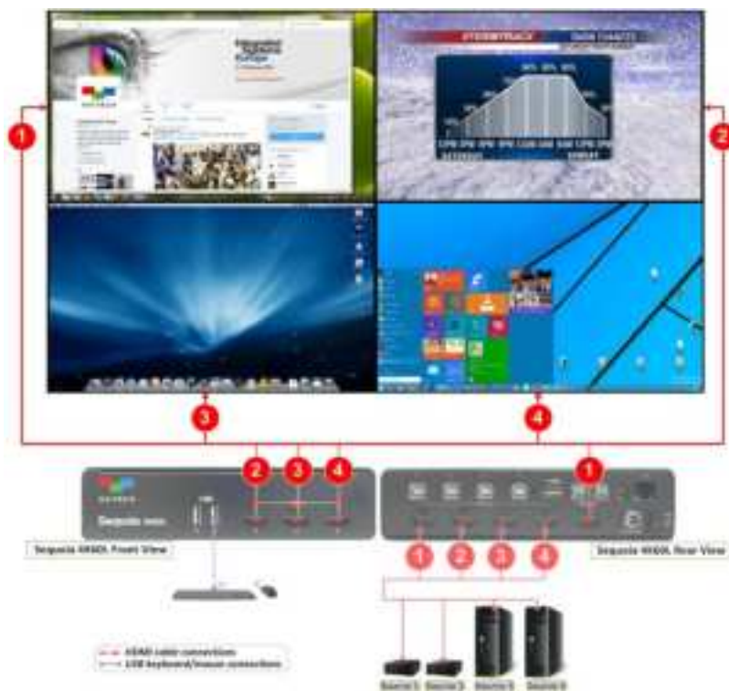
Figure 2.3.1 Sequoia 4K60L Video Wall Connection Diagram
