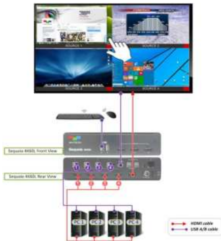
Figure 6.1.1 Sequoia 4K60L with Touch Screen Connection Diagram
