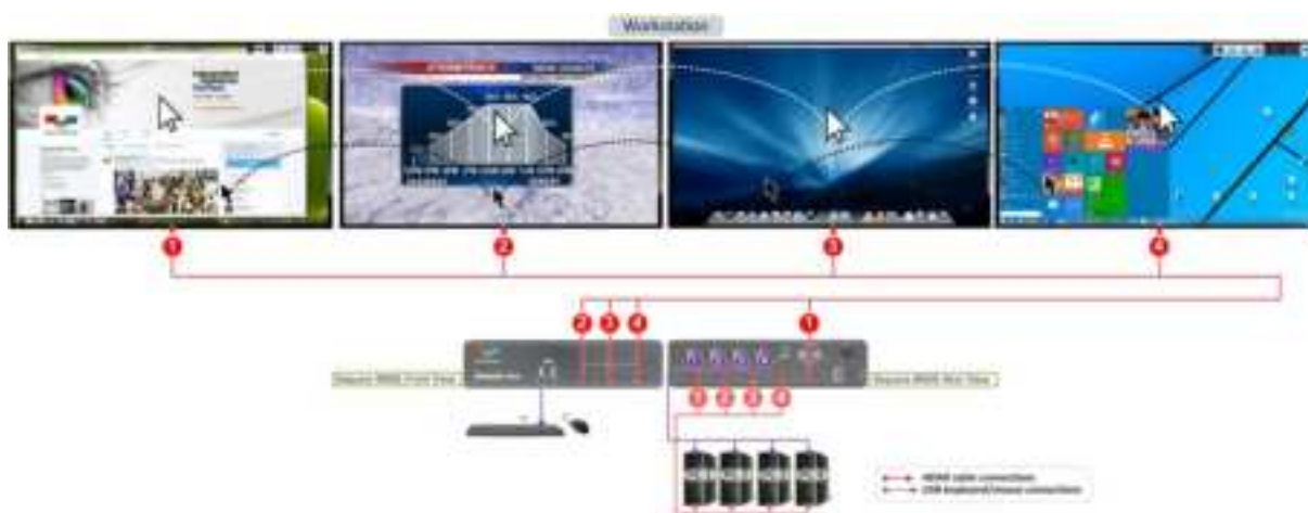
Figure 2.2.1 Single-View Seamless Switching Connection Diagram
