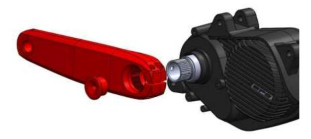
Use the **6mm hex torque wrench** to tight the axle screw to 2Nm, tighten then the two radial bolts with a **5mm hex torque wrench** to 14Nm. Repeat for both sides.
