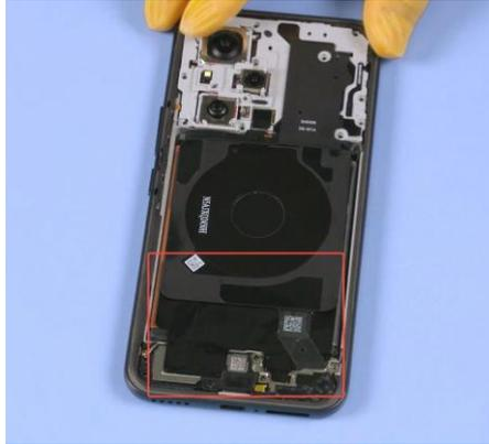
4. Use the tip of the Phillips screwdriver to tighten the 20 M1,4 screws.
