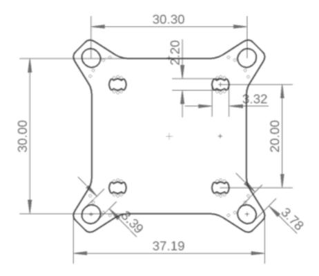
Maximum outside dimensions:  $37,2 \times 37,2 \text{mm}$ , without outside tips  $30 \times 30 \text{mm}$  Mounting hole arrangement:
