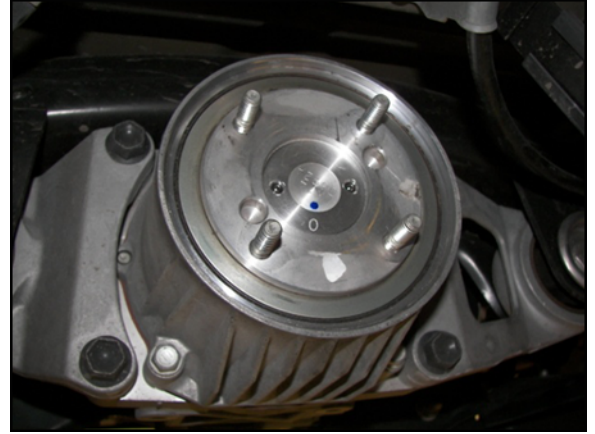
Figure 2. For This Deflector Type, Use P/N 41252-42013
