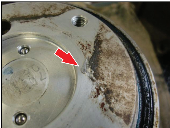
Figure 6. Damage Where Propeller Shaft Contacts Coupling Body
