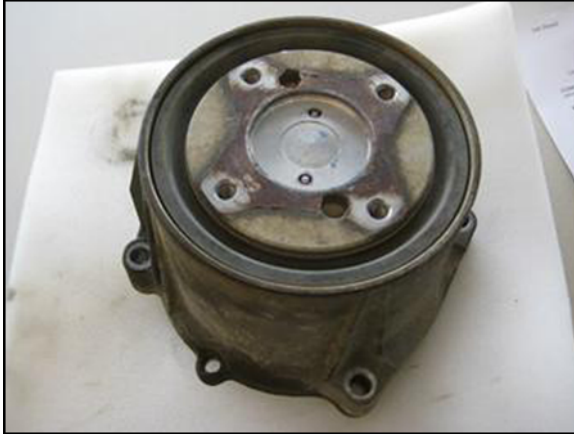
Figure 1. For This Deflector Type, Use P/N 41252-42020
