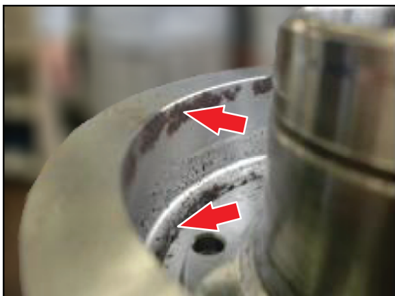
Figure 8. Rust/Corrosion on Inside of Coupling Body
