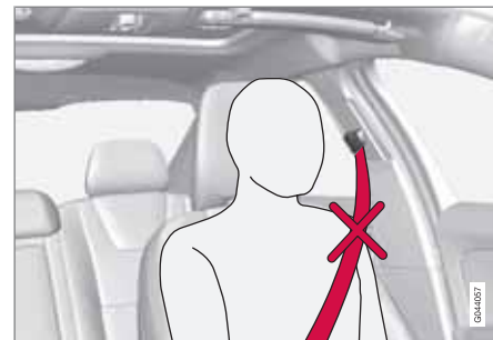
Incorrect height adjustment
