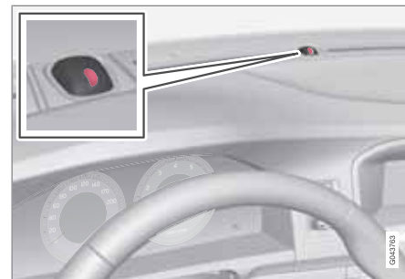
Lock/alarm indicator light
