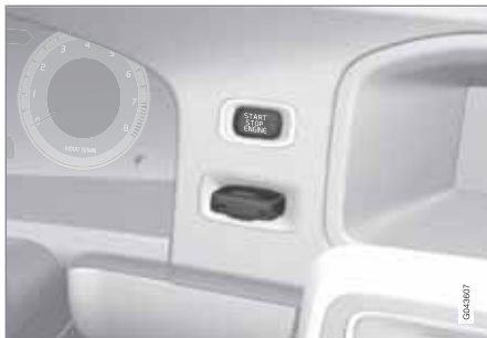
Ignition slot with remote key inserted and START/STOP ENGINE button.
