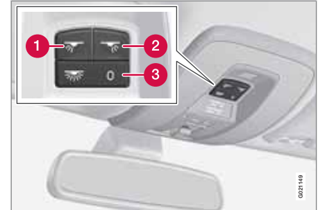
Light switches, front roof lighting
