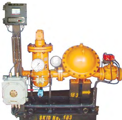
MSA meter skid with Toptech SMP controller
