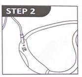
Before turning on the lights, charge the magnifier using the provided USB charging cable to ensure proper functioning of the lights Red: Charging
