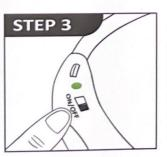
Please turn on the battery switch after charging to activate the light button function, which serves to prevent inadvertent activation and conserve power.
