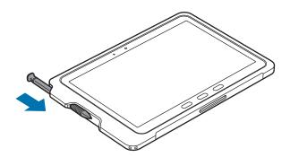
① Do not insert the S Pen backwards into the protective case.
