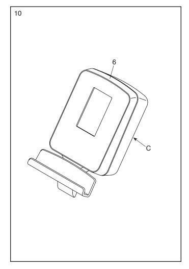
11. Have a second person hold the Console (6) near the Handlebar (5). Connect the Main Wire (87) to the receptacle on the back of the Console.
