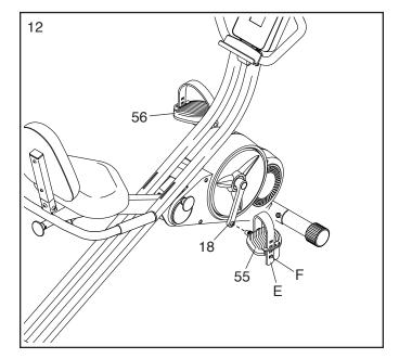
13. After the exercise bike is assembled, inspect it to make sure that it is assembled correctly and that it functions properly. Make sure that all parts are properly tightened before you use the exercise bike. Extra parts may be included. Place a mat under the exercise bike to protect the floor.
