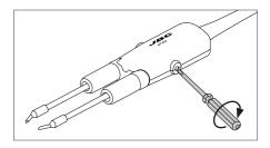
Lock the fixing screws.
