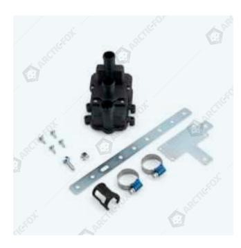
Calix Forced Circulation Heater (FCH) is a hose mounted engine block heater with an integrated circulation pump that spreads the heat faster and more evenly in the engine, making it more efficient. Additionally, the FCH is easier to install compared to a heater with a separate circulation pump as FCH is more flexible in the positioning of the heater.
