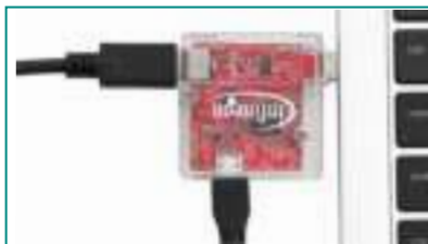
Step 4 USB-PD source and sink connected to CY4500-EPR
